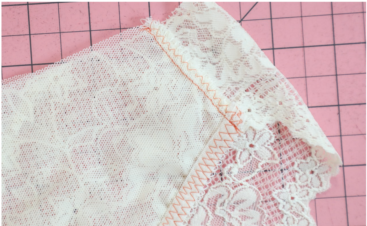
Seam finished with zigzag stitch
