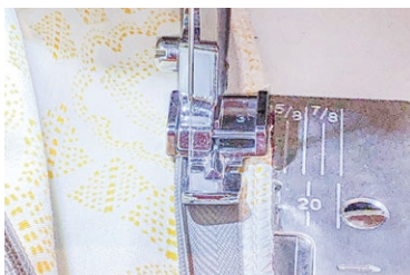
Sew zipper in place on skirt front piece.
