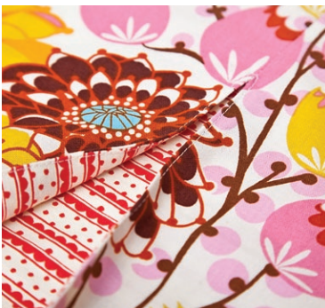
Edgestitch pleat edges on right side of fabric.
