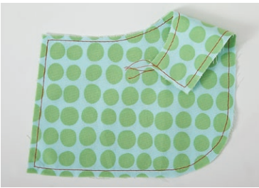
Baste pocket front and lining together.
