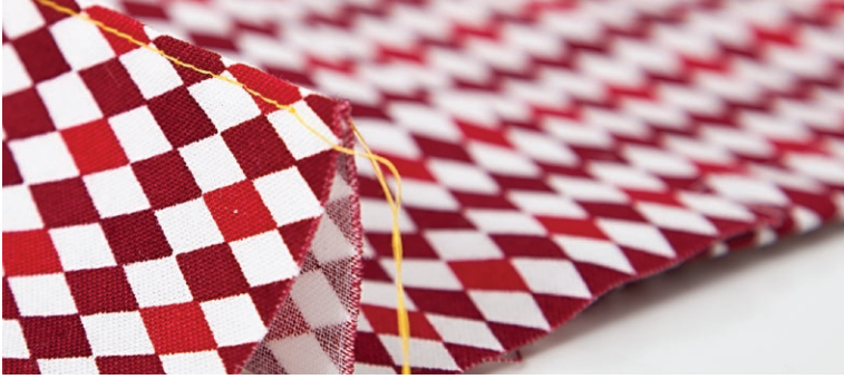
Finished edgestitched folds
