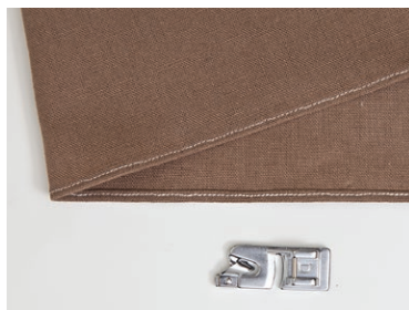
Example of rolled hem on ruffle
