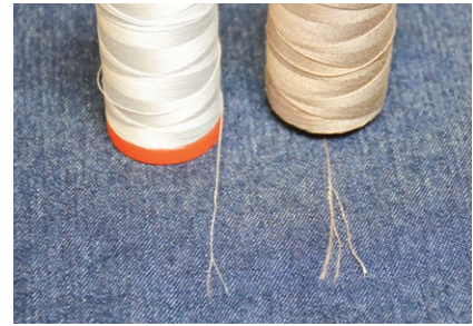
2-ply versus 3-ply thread
